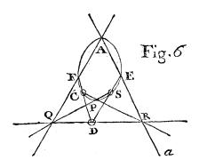
with each of them being carried over a fixed Right Line, their Intersection with each other describes the Locus, which is shewn to be a Conick Section. The Intersection of QDR with SQ, is supposed to be carried over the fixed Right Line AF; the Intersection of the same QDR with CR, is supposed to be carried over the fixed Right Line AE; and in the mean time, the Intersection of the Right Lines SQ, CR, that revolve about the Poles S and C, describes a Conick Section.
