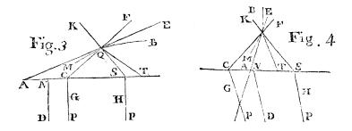
Constitute the Angle S Q T equal to C Q A, as before, and let Q T meet C S in T. Take C N equal to S T, the opposite Way from C that S T lies from S. Through N draw D N parallel to C G or S H, which are now parallel to each other, and D N shall be an Asymptote of the Curve described by the Motion of P.
